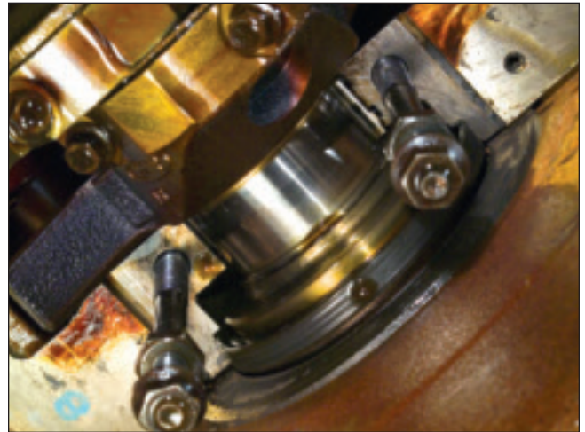
A closeup view of the rear main crankshaft journal. No visible wear detected.
