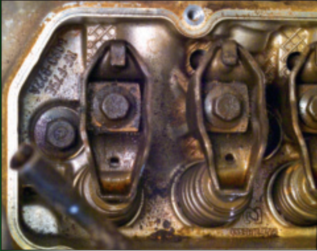
The head and rocker arms were very clean and free of heavy deposits. Note that you can still see the honey-comb stamping and manufacturer's part number. This is normally an area of the engine where you would see heavy varnish deposits with a conventional engine oil.
